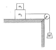
Mech. 3. Block 1 of mass  $m_1$  is placed on block 2 of mass  $m_2$ , which is then placed on a table. A string connecting block 2 to a hanging mass M passes over a pulley attached to one end of the table, as shown above. The mass and friction of the pulley are negligible. The coefficients of friction between blocks 1 and 2 and between block 2 and the tabletop are nonzero and are given in the following table.
